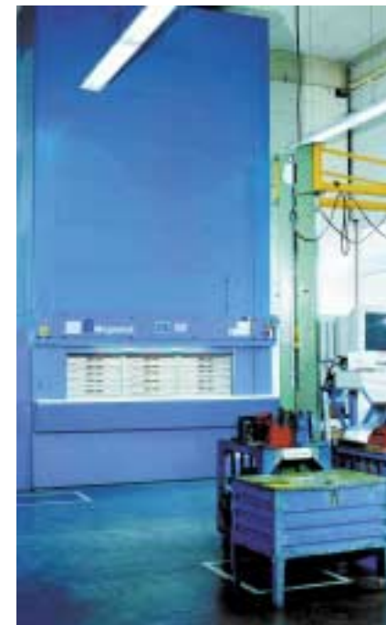
Vertical Carousel in production- and assembly-area
