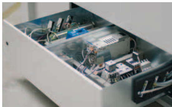
Easily accessible drawer for the control electronics
