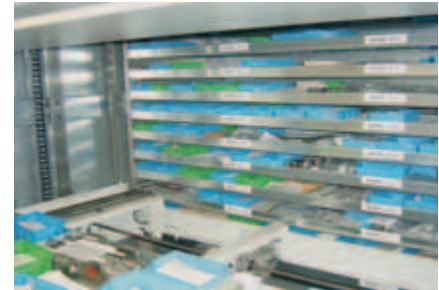
Compact storage in lift shelves provides additionally required space.
