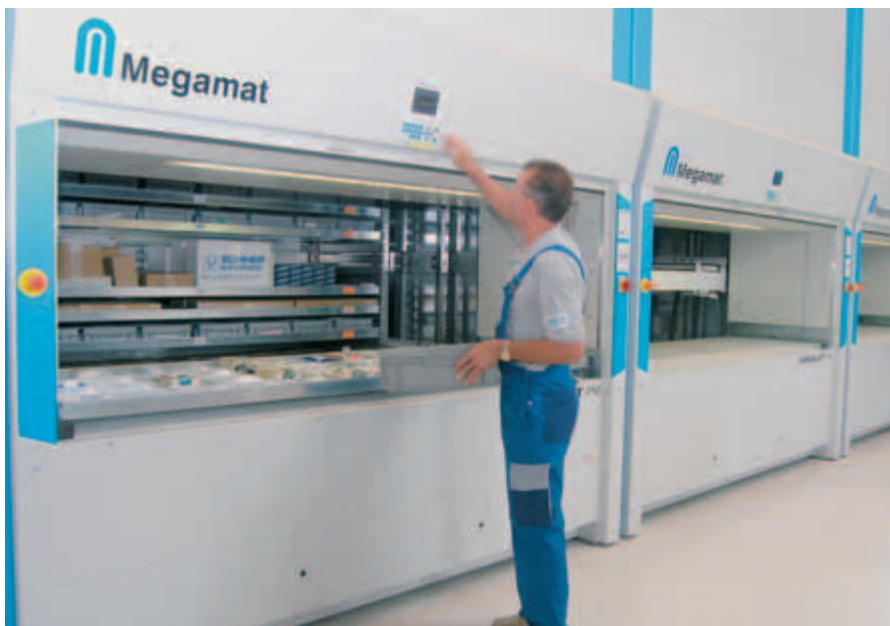
Megalift combination as a commissioning store with direct data link to order handling
