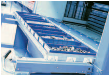
Docking station for trolley. Complete trays can be transported in this way.
