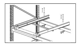
4. The upper frame is then attached by pulling the unit through the C profiles from the rear. This is then lowered carefully onto the lower frame.
