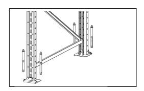
2. Both the front and rear beams need to be rigid, we recommend to bolt the beams to the upright. This needs to be done at the front and back.
