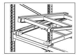
5. Once on the lower frame, the bent flange prevents the pull out rolling backwards out of the C profile.
